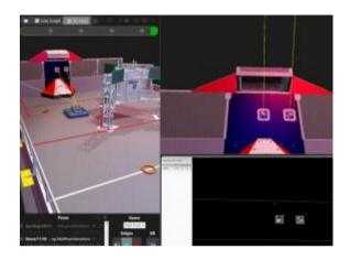
We implemented a custom filtering algorithm to reject invalid AprilTag observations caused by dirty camera images, along with a Kalman filter to fuse vision and odometry data.
