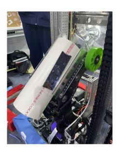
During testing, we found out that the CORAL sometimes gets stuck in the wheeled transfer system. Which we added a guiding board to help push down the CORAL in place for a successful intake.
